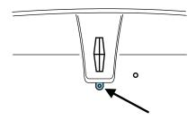
To use the camera system, place the transmission in R (Reverse); an image will display on the navigation screen. The area displayed on the screen may vary according to the vehicle orientation and/or road condition.
